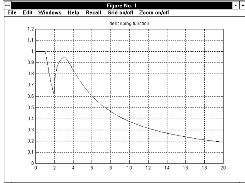
Figure 3.13. The describing function of the nonlinear element in Fig. 3.12.
