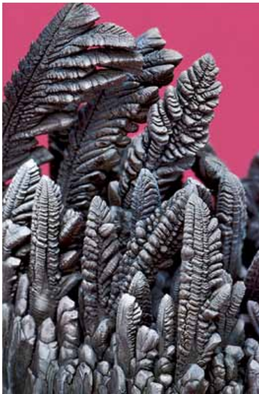
Figure U.2 Metallic dendrites formed during electrochemical deposition. Such dendrites occur in the rapid discharge of a lead storage battery and can lead to an internal short circuit.
