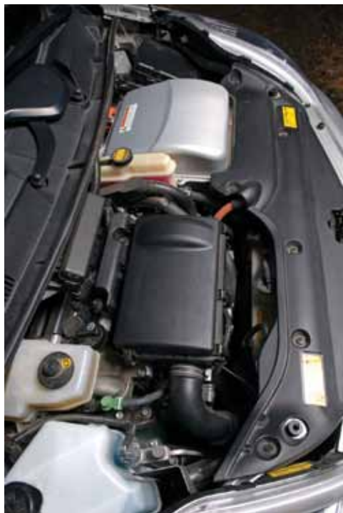
Figure U.3 Hybrid cars contain both a gasoline and an electric motor. NiMH batteries are charged while braking by spinning the electric motor in reverse, making it act as a generator. The stored energy is then used to supplement the gasoline engine when accelerating. In this way hybrid cars can achieve fuel efficiencies significantly greater than those of conventional vehicles.
