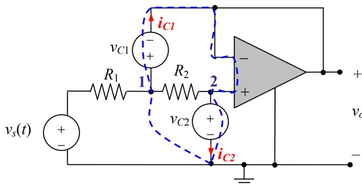
LKC nodo 1:  $i_{C1} = \frac{v_s - v_1}{R_1} - \frac{v_1 - v_2}{R_2}$
